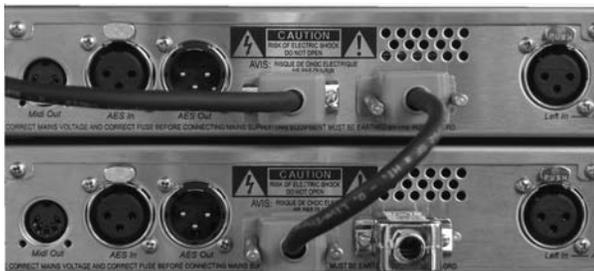
To connect more M7 to the chain, just loop from one to the next and terminate the last one. The order in which the units are connected will determine the machine number sequence when using them from the M10. First machine is #1, second one is #2 and so on up to 8.
